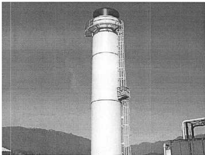
Exhibit 9. The Dock Is Equipped With H 2 S Scrubbers (Left) And Oil Loading Arms (Right)
