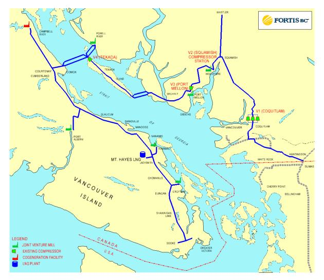
Figure 5-1: Layout of the FEVI Transmission System
