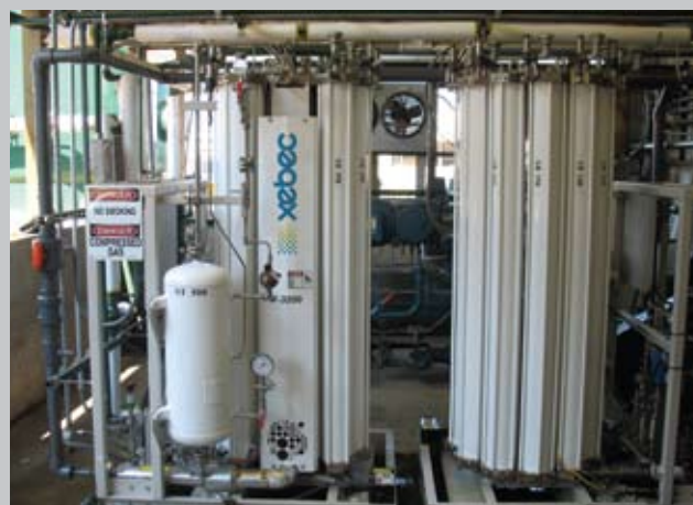
XEBEC M-3200 processes dairy farm biogas for distribution to customers via Michigan Gas Utility natural gas pipelines.
