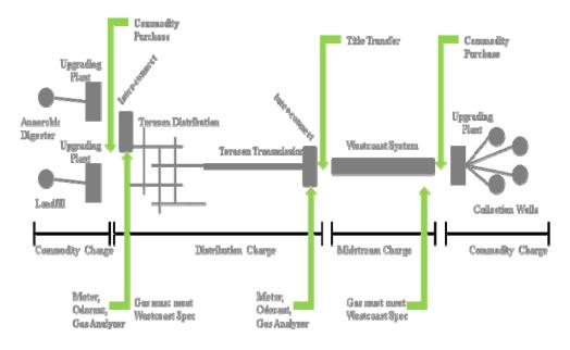
Figure 8-4: Structure of Natural Gas Supply Chain with Biomethane
