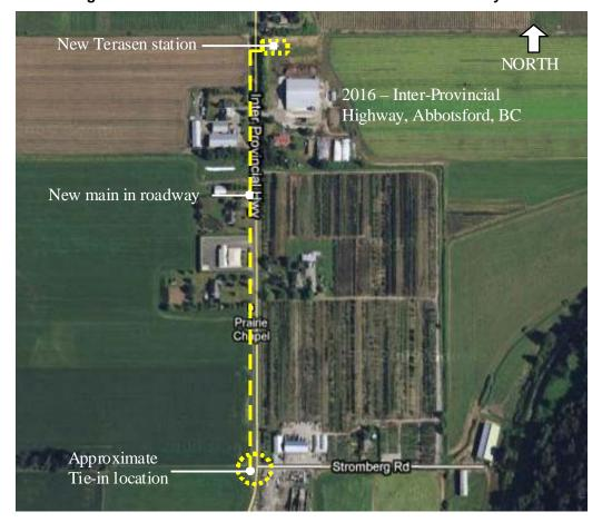
Figure 9-6: Connection Point to Terasen Gas Distribution System
