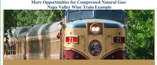
The Napa Valley Wine Train started a program for the experimental conversion of a Napa Valley Wine Train Alco locomotive to 60% natural gas and 40% diesel fuel mixture. In 1999 the conversion became permanent. A total conversion of locomotive 73 was completed and it was put into service using 100% Compressed Natural Gas on in 2008.
