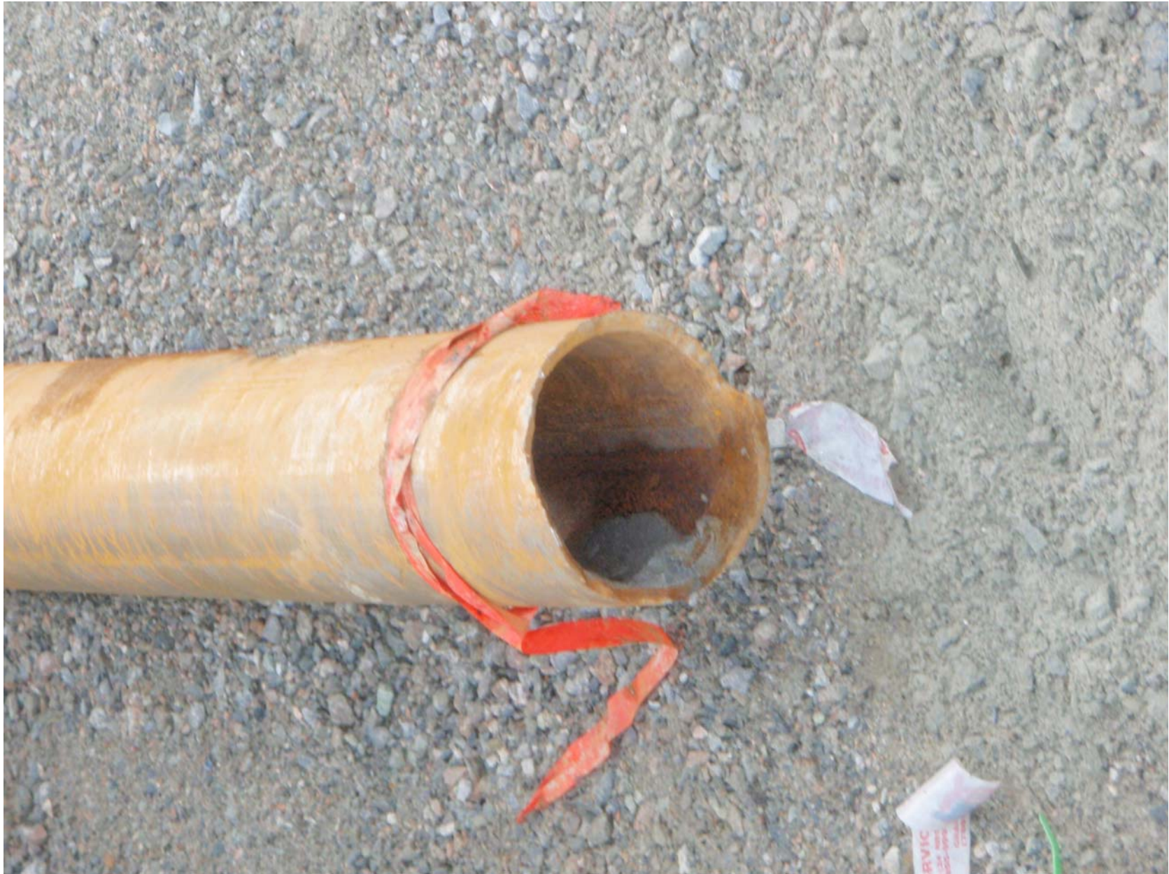
Jan 2, 2010. NPS 20 HDD failure. XXH NPS 6 drill pipe “twist-off.”
