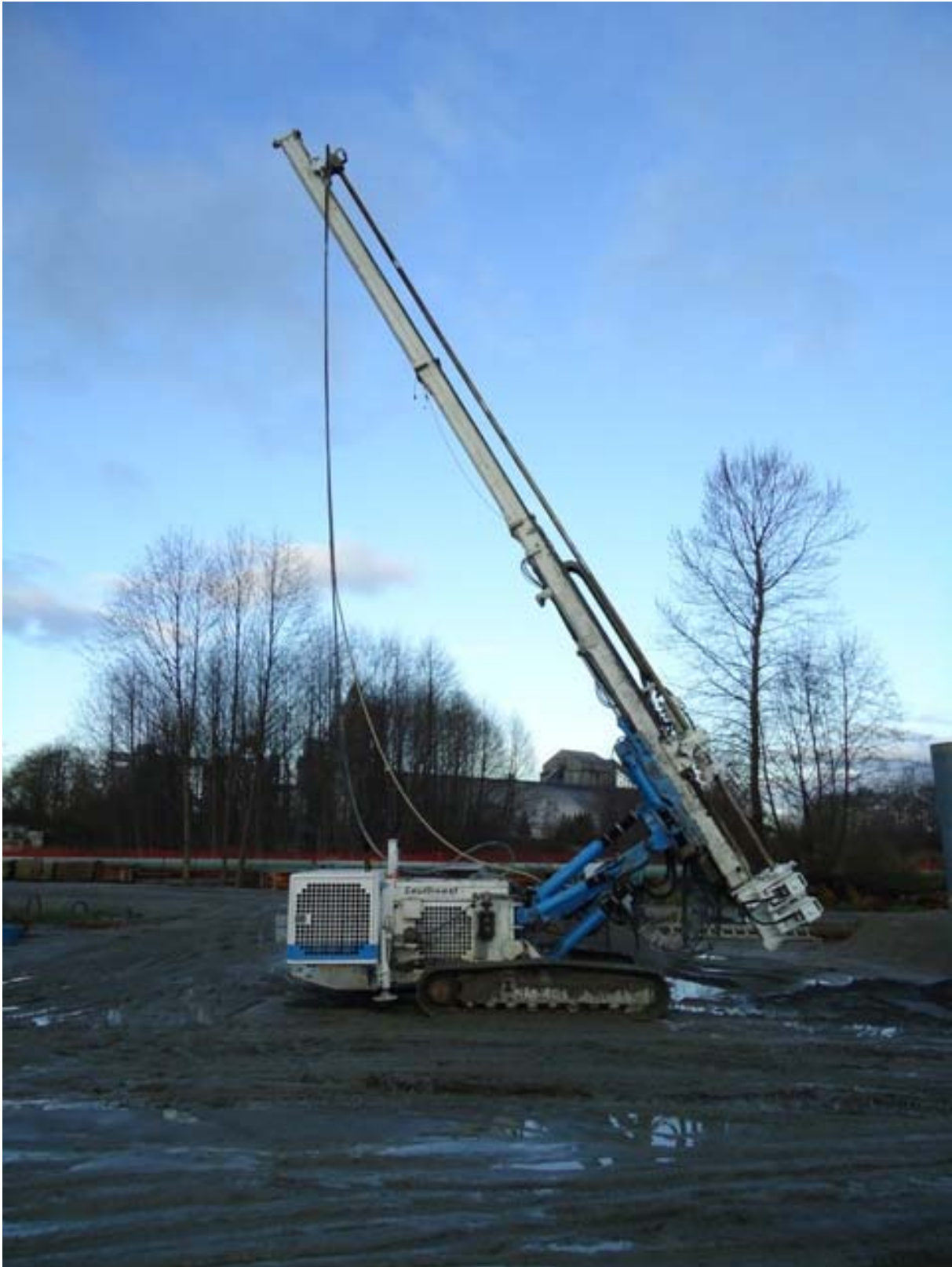
Mar 27, 2011 – Jet grouting rig
