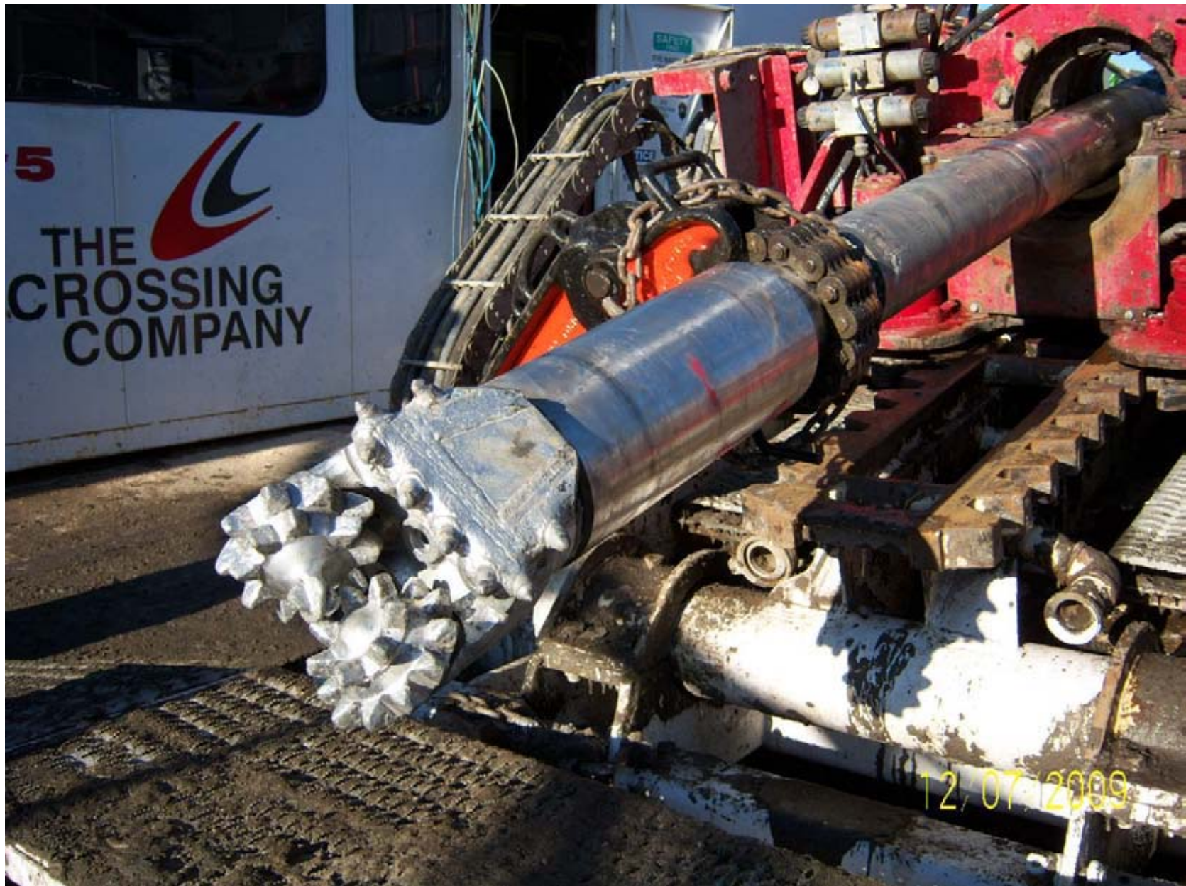
Dec 7, 2009. North Side HDD Rig - steerable jetting drill bit.
