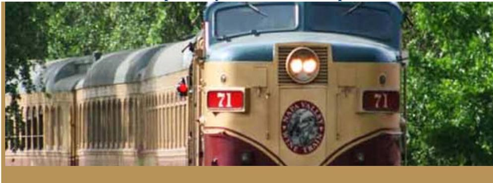
The Napa Valley Wine Train started a program for the experimental conversion of a Napa Valley Wine Train Alco locomotive to 60% natural gas and 40% diesel fuel mixture. In 1999 the conversion became permanent. A total conversion of locomotive 73 was completed and it was put into service using 100% Compressed Natural Gas on in 2008.
