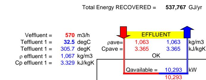
Energy to be Removed from Effluent prior to Discharging = 394,250 GJ/yr
