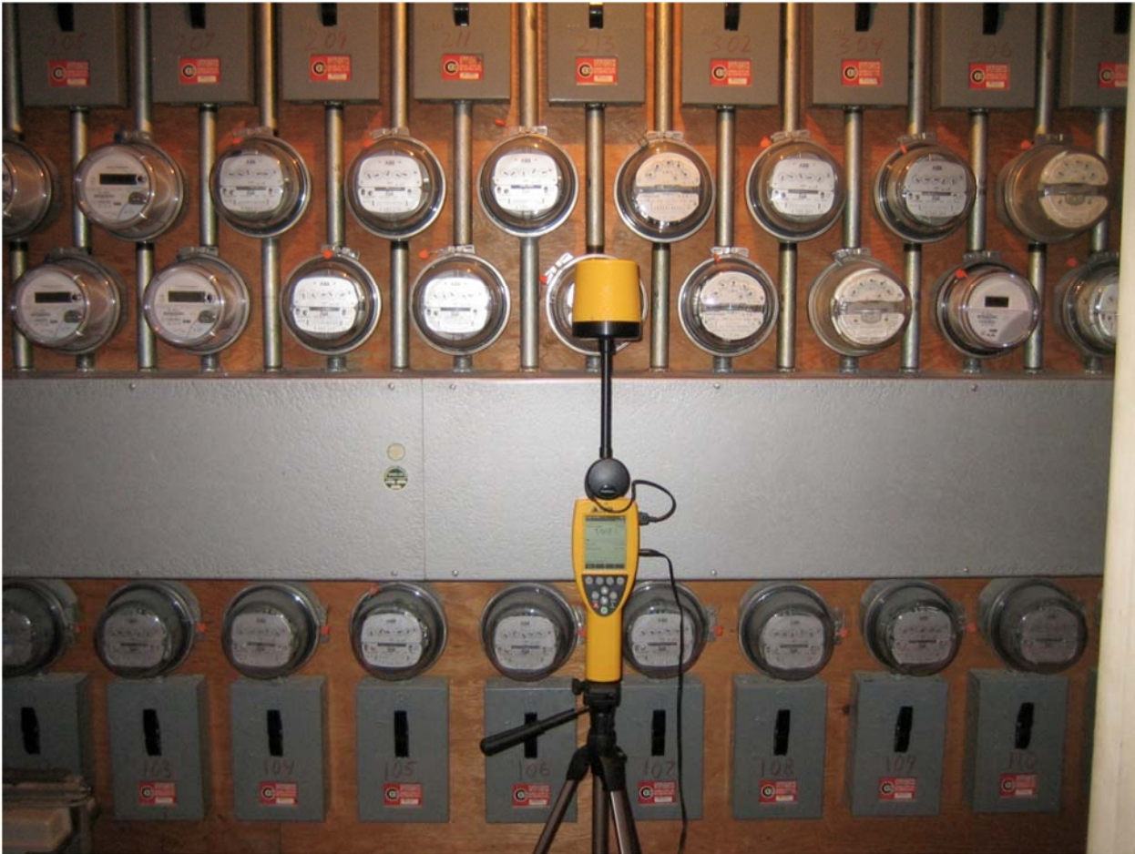
Image 1. Test setup depicting the elevation of test meter with respect to Itron electrical meters. The test meter is centered within the bank at an approximate elevation of 1.8m.
