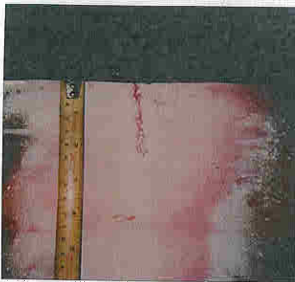
Crack at Bucket #9 outside view before gouging
