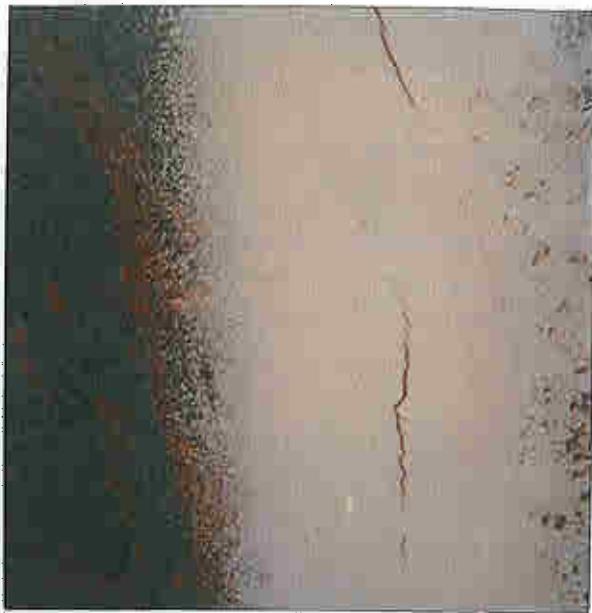
Bucket #5 - Two cracks - Total length of 10"
