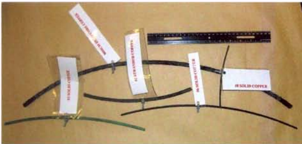
Figure 21: Single pieces of both stranded and solid copper conductor samples with identification. Stranded conductors were a 90 MCM hemp core (6 strands), and a #2 stranded conductor (7 strands), solid conductors were #8, #6 (6c), #3 (3c) and #2
