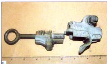
Figure 3: Hot tap disassembled for examination
