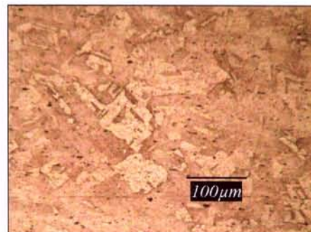
Figure 12: Microstructure 0.500 inches away from fracture surface Hardness 60 HV Mag: 200X
