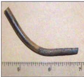
Figure 5: Section of failed #4 AWG conductor removed from hot tap
