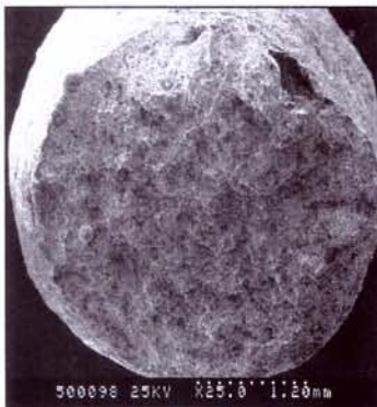
Figure 8: Low magnification scanning electron micrograph of fracture surface of copper conductor.
