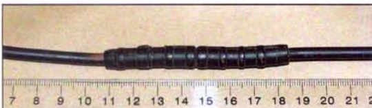
Figure 24: Macro image of compression splice on sample 4b. Note corrosion product on surface of conductor and splice
