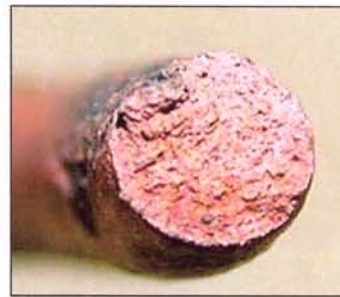
Figure 6: Macro image of fracture surface of copper conductor
