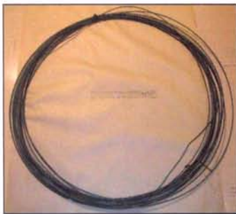
Figure 18: Coil of #6 AWG copper conductor received for examination, identified as sample 6A
