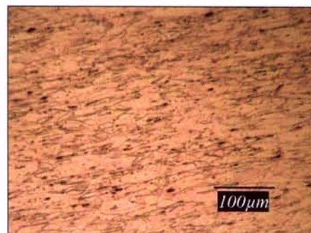
Figure 32: Microstructure seen in sample 4b within splice area. Magnification: 200X
