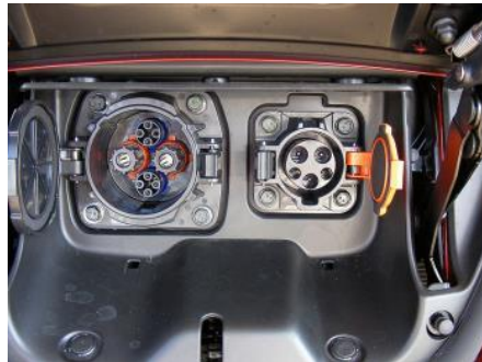
Figure 28: Nissan Leaf charging ports, left to right: CHAdeMO DCFC, J1772 AC
