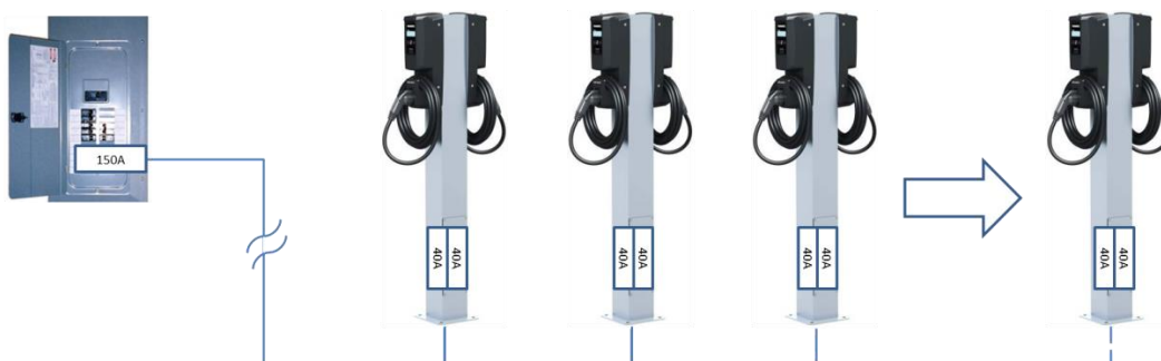
Figure 35: AddÉnergie's PowerSharing system enables expansion of EVSE installations using a daisy chain configuration
