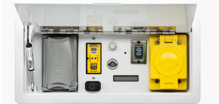
Figure 38: Export power panel on a VIA Motors V-Trux with 2x120V and 1x240V outlets
