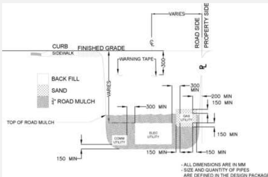
Figure 1: Joint Trenching
