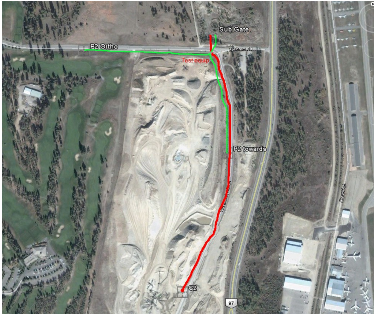
Figure 2 Ground Impedance Measurement Configuration
